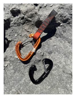
The broken quickdraw from the Mickey's Beach incident. The wire gate has been fixed in the open position, indicating that it was loaded while not engaged with the gate notch.
