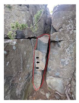
The failed cam placements in the rappel anchor are marked. Although it appears to be comprised of stacked blocks, the pillar is one solid block. However, the entire pillar moved under load.
