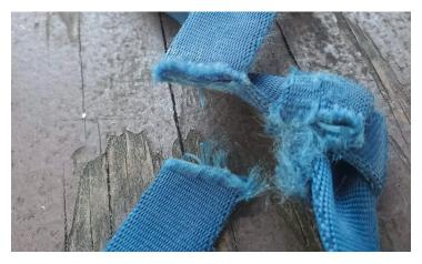
This sling was tied to create a masterpoint loop for a top-rope anchor. The loop apparently rubbed against a sharp edge and cut.
