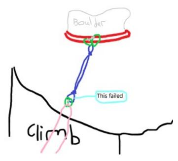
Sketch of the anchor set-up atop Gill's Nose, showing where the masterpoint loop rubbed against the sharp edge of the cliff top.
