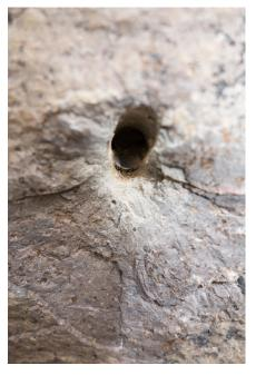
The third bolt hole on Life in Electric Larvae Land. The rear half of the bolt can still be seen embedded in the rock. The rock scarring below the hole is likely at least partially from the installation of the bolt, but may have been enlarged during the bolt failure.
