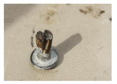
The fractured third bolt from Life in Electric Larvae Land. Note the corrosion below the surface of the bolt head.
