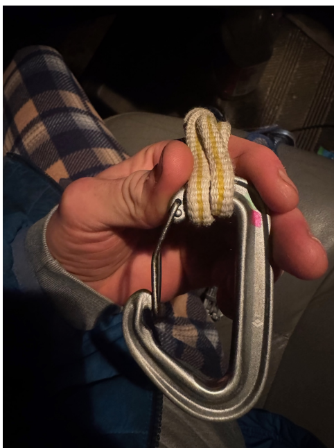
The alpine draw. If one looks closely, the displaced wire gate is visible.
