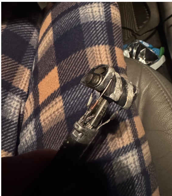
Ogle's No. 0.4 Z4 missing a chunk of an inside cam.
