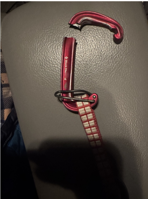
One of the damaged/broken carabiners.
