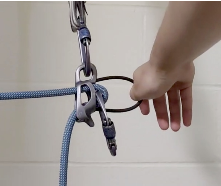
Fig. 2: This shows how the ATC orientation can potentially allow the rope to run through the device in guide mode.
