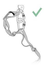
After suffering his near-fatal fall, Laycock wrote to ANAC: "To shorten my PAS at an anchor, I won't unclip the first (longest) loop anymore. I'll clip an additional locking carabiner in the shorter loop, then clip it to the first locker. Previously, and in the case of my accident, I completely unclipped from one loop and reclipped the closer knotted loop."
