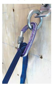
Laycock's jammed knot accident was virtually identical to another in Arizona in 2021. In both cases (and in this re-creation), a tether carabiner of the same make and model had a bottom basket flat enough and shaped in such way as to allow a jammed knot to hold weight, if only for a few moments.
