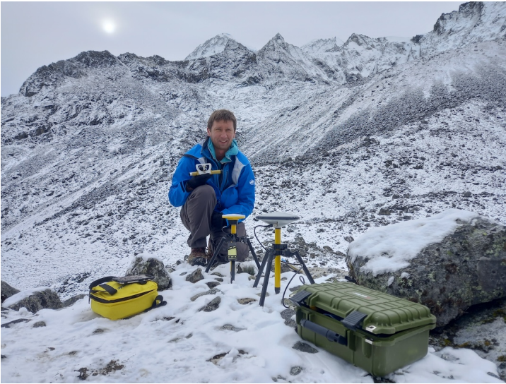
Eric Gilbertson with the survey equipment set up at base camp: an Abney level, Promark 220 dGPS with Ashtech antenna, and DA2 dGPS. Pico Cristóbal Colón (left) and Pico Simón Bolívar (right) are visible in the background.
