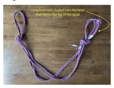
An accident involving a quad anchor system occurred when a climber clipped the loop formed by unusually long knot tails that had been tucked into a knot. When weighted, the tails slipped out of the knot.
