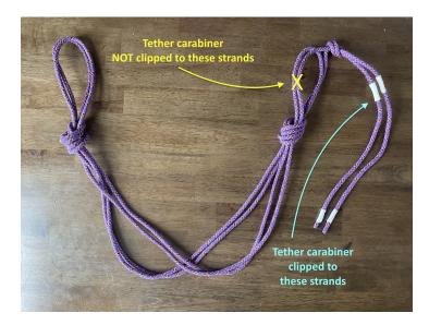
An accident involving a quad anchor system occurred when a climber clipped the loop formed by unusually long knot tails that had been tucked into a knot. When weighted, the tails slipped out of the knot.
