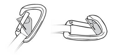
It's an unsettling thought, but carabiners can, on rare occasion, unclip from bolt hangers. When the bolt is clipped from right to left and the hanger angles down to the right, tension on the quickdraw can raise the carabiner and lever the gate open. Foster Denney
