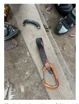
The bolt-end carabiner of this quickdraw broke in a leader fall, most likely when the gate improbably "nose-hooked" a glue-in, rod-stock-style bolt.
