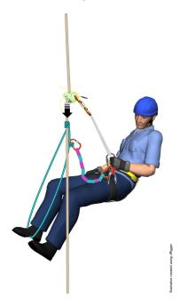
As the progress-capture device slid onto the top of the prusik, it caused the hitch to fail and the climber slid down the rope to the ground.
