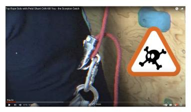
Clip from a video demonstration showing how the Shunt can flip upside down and catch the rope in such a way that it releases under load. Heed the manufacturer's instructions: Do not use the Shunt as a solo top-rope device.
