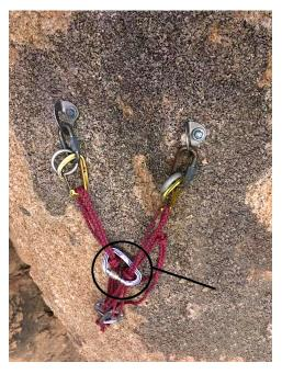
The anchor atop Owl Rock after the accident, showing the carabiner the climber failed to clip correctly when shortening his tether (the upper carabiner, clipped to the shelf on the cord).
