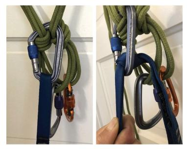
Reconstruction of the anchor atop Owl Rock. The climber first clipped in with the end of his tether sling (left). He then tried to shorten his tether by clipping a shorter loop created by an overhand knot tied in the sling. However, he failed to capture the shorter loop (right). Under load, the knot initially jammed in the base of the carabiner. It temporarily held his weight, but then pulled through.
