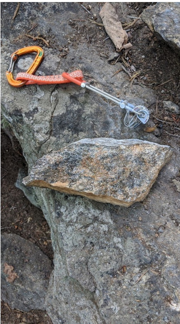
The cam and a piece of the flake that broke during a fall at Melrose Mountain.
