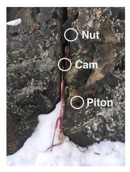
Post-avalanche view of the anchor on Pioneer Peak. The anchor remained mostly intact; only the cord connected to the piton had failed.
