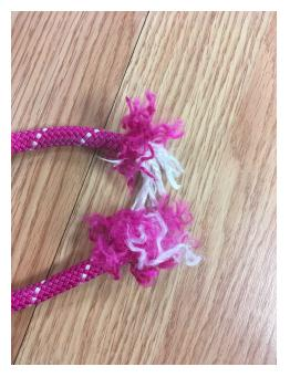
The rope that cut on Pioneer Peak likely failed when it sawed against a sharp rock edge by the anchor.
