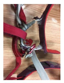
Damage to one climber's harness sustained as she was hit by avalanches at a rappel stance on Pioneer Peak. The harness likely would have sustained many kilonewtons of force to be damaged this way, yet both it and the anchor held. Ultimately, the climbers concluded, a screw-gate locking carabiner must have unlocked and detached itself from the anchor during the chaos of the avalanches.
