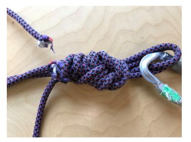
Detail of a compromised cordelette at an anchor above a Smuggler's Notch ice climb.
