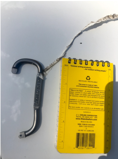
The spine of this carabiner was clearly marked "Not For Climbing," but the words were covered with tape. The carabiner broke during a climber's fall at the Pit near Flagstaff.
