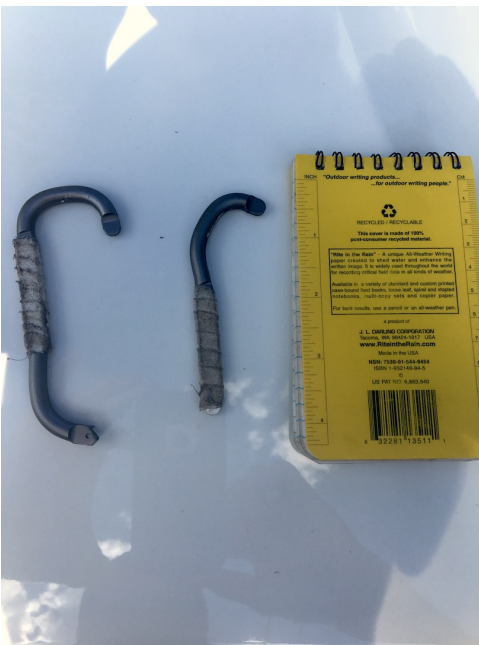
Tape covering the spines of carabiners that broke in an accident at the Pit.
