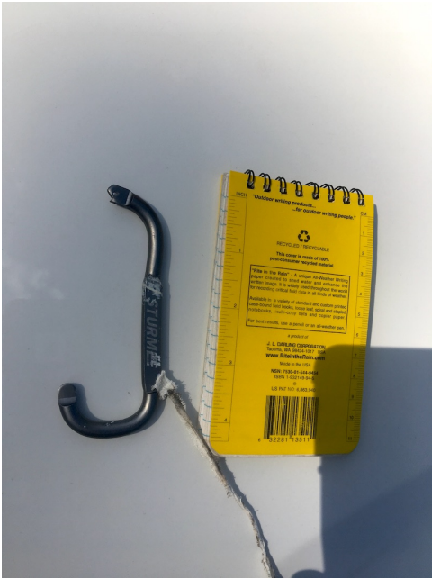
One side of a carabiner that broke in an accident at the Pit, near Flagstaff.
