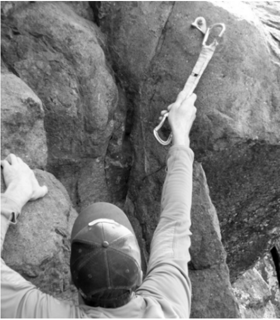
A homemade "stiff draw" being used to clip an out-of-reach bolt hanger.
