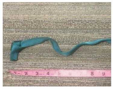
A 9/16-inch sling with an overhand knot, found with the climbing guide who fell from the Owen-Spalding rappel on the Grand Teton. Investigators concluded this sling, used to tether the guide at the rappel anchor, had been tied with a water knot that came undone under load.
