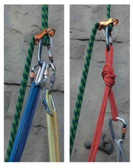
[Left] Mockup of the rigging used to rappel with a haul bag in this incident. The locking carabiner clipped to the yellow slings (connecting the haul bag to the rappel carabiner) is believed to have unclipped. Including the haul bag connection (not shown), this setup used seven carabiners. [Right] A much simpler setup with a doubled cordelette to connect the rappel device to both the climber and the haul bag (gray slings), using only two carabiners.
