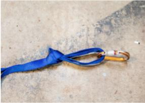
Correctly tied BHK, with extra "ear" of webbing (lower loop in photo) clipped to the master point for safekeeping. (Middle) Incorrectly tied master-point knot, creating a slipknot with no backup. (Bottom) Under load, the extra ear of the slipknot pulls through and the knot fails.
