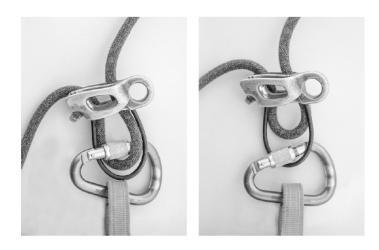
[Left] A belayer's screw-gate carabiner was unlocked by the action of the rope as he lowered his climbing partner. [Right] The rope then popped out of the open gate.
